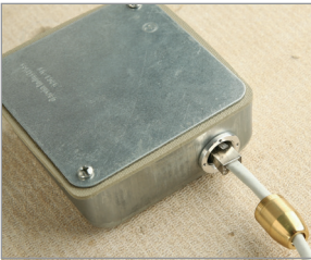
Fig G. Fasten the lid 3 on top of the junction box. Insert RJ45/Cat cable into JBM3 receptacle. (See back page for installing seismic cable)
