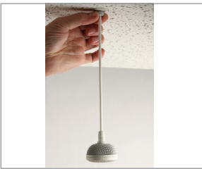
Fig J. Position the microphone by turning the cable as necessary and gently turn the nut clockwise to secure (1 to 2 turns). Do not over tighten.
