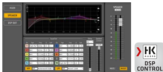
Screenshot of the remote DSP CONTROL software. You can download this software free of charge at the LINEAR 7 product page at www.hkaudio.com . The speaker and DSP Out parameters are identical, but the powerful onboard DSP lets you configure each set independently.
